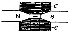
FIG. 25.—DIAGRAMMATIC REPRESENTATION OF THE BLONDEL MOVING IRON OSCILLOGRAPH
